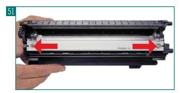
**33** Install the MRS assembly. Make sure the clear strips from the doctor blade ride on top of the magnetic roller (see Figures 52 and 53).
