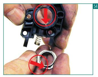
35 Install the holder, two screws and spring. Make sure the screw holes line up, and that the two locking tabs on the bottom of the holder are in the correct place. This can be tricky to get in place until you've done it a few times. Take your time and don't force the fit (see Figures 55 and 56).
