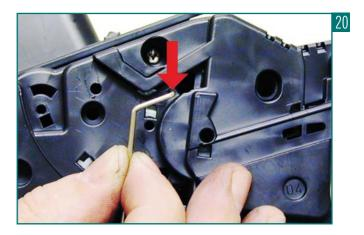
3 On the opposite side of the cartridge, carefully pry off the drum cover plastic arm. The spring will probably pop off - take care not to lose it. We will go over the installation at the end of this article. Remove the drum cover assembly (see Figure 21).
