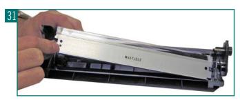
14 Due to the high speed and page counts of these cartridges, we recommend that the wiper blades be replaced. Make sure that the wiper blade foam seals are clean (see Figure 32).
