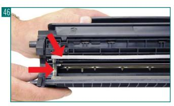
28 Note also the new heavy-duty style magnetic roller contact. This, when combined with the new larger diameter of the roller, allows the cartridge to run at the higher speeds that these machines are capable of (see Figure 47).
