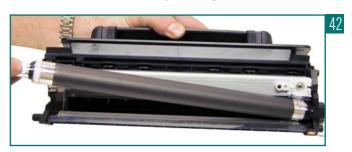
25 Remove the two doctor blade screws and the doctor blade. Note the clear plastic strip that covers the doctor blade screws. Slide the screwdriver under the strip. Be careful not to damage the strip (see Figures 43 and 44).
