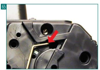
44 Install the arm onto the cartridge. Pull the arm fully back to release the spring from the notch. Check to make sure the drum cover operates properly (see Figure 66).
