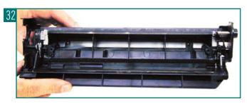
15 Install the new wiper blade and two screws (see Figure 33).
