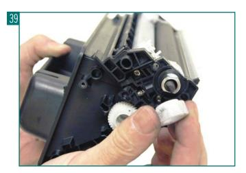
23 Note the location of the spring that sits between the MRS holder and the hopper. Remove the two screws, spring and the holder (see Figures 40 and 41).
