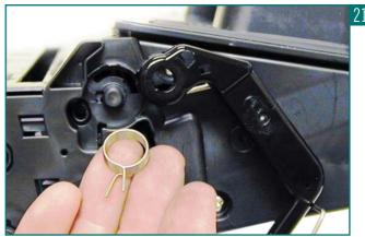
4 Remove the metal bar from the left side, and remove the entire drum cover assembly. Make sure you put the spring in a safe place (see Figure 22).
