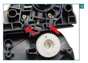
36 Install the magnetic roller drive gear. Make sure the bushing part of the gear faces into the cartridge (see Figures 57 and 58).
