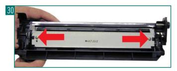
**13** Remove the wiper blade from the cartridge, and clean out the waste toner (see Figure 31).
